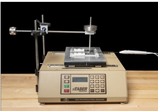
To simulate aggressive use, a weight was added to the test machine weight holder so the 20° angled stylus applied a 7 N load at the point of contact on the probe. The stylus on the counterbalanced arm of the
