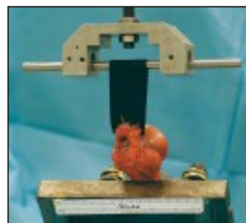
Figure 3: Position of a repaired humerus for mechanical testing.
