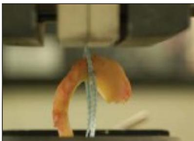
A preload of less than 2N was manually applied to the meniscus, and each sample was cycled from 5-20N at 1Hz for 1000 cycles. Following cycling, a load to failure was conducted at 12.5 mm/sec, as per testing reported by Zantop, et al (2005). For each sample, the displacement after 1 cycle, 100 cycles, and 1000 cycles, the ultimate load, and the mode of failure were recorded.
