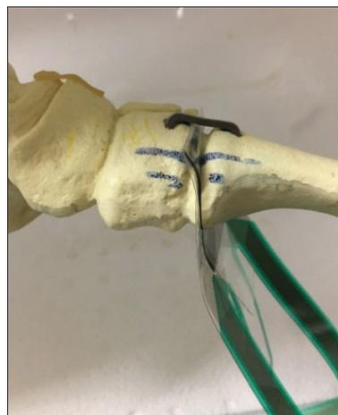
*Forefoot bone stimulation model showing placement of pressure sensor to measure compressive force of implant. Note: Excess metatarsals removed from models.*
