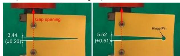
Figure 2: Experimental test setup with mounted sharp cutting edge (left) and hinge pin (right) specimen.
