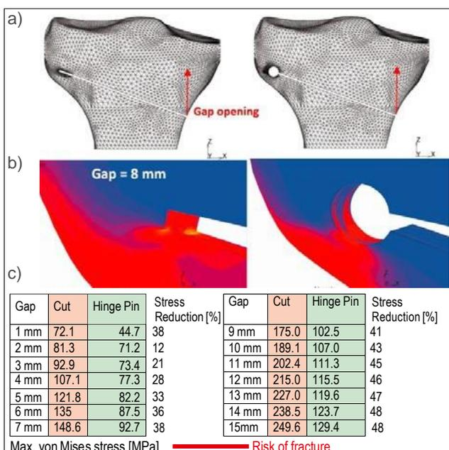
Figure 1: FEA models (a) with von Mises stress results over the gap opening (b/c).
