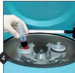
**4** Place the syringe into one bucket and an appropriate counter balance in the opposite bucket. Two syringes may be used to increase dosage.
