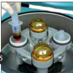
**5** Run the centrifuge at 1500 rpm for 5 minutes. Remove the syringe, taking care to keep it in an upright position to avoid mixing the plasma and red blood cells.
