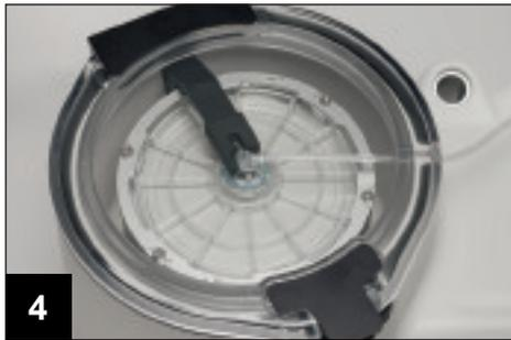
4 Place the tube leading from the separation chamber through the centrifuge well slot. Close the centrifuge lid.
