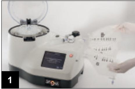
1 Turn on the Angel System. Open the centrifuge lid cover and lift the centrifuge stator arm. Remove the Angel Processing Set from the tray and place it on top of the machine.
