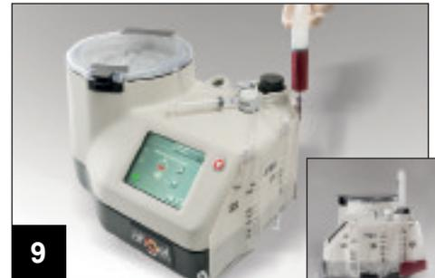
9 Inject the anticoagulated aspirate into the "Whole Blood In" chamber. *Note: The minimum processing volume required is 40 ml of anticoagulated whole blood. The ratio of whole blood to citrate anticoagulant (ACD-A) is 7:1.*
