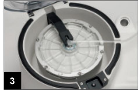
3 Once aligned, press down and turn clockwise until the position indicators snap into place. Lower the centrifuge stator arm and align it with the raised tab on top of the separation chamber.
