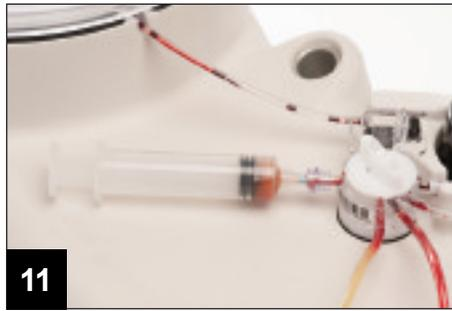
**11** The first component to be collected is platelet-poor plasma (PPP). The Angel System will then adjust the valve position to collect PRP until red blood cells are detected and the preset hematocrit is reached.
